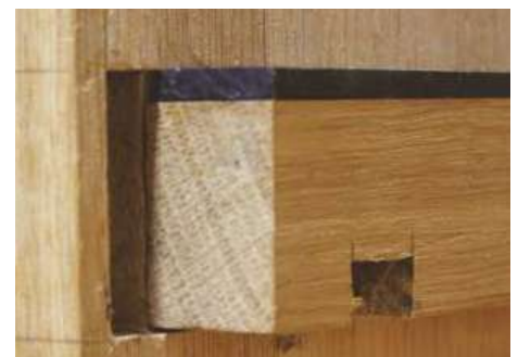
▲ Pic 14 Both lopers have a thin strip of oak along their top edge. There is a brass adjuster screw recessed underneath
